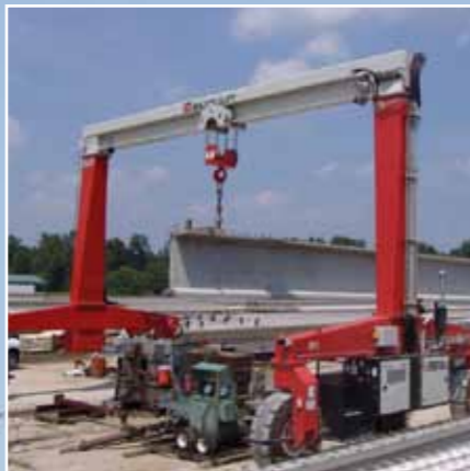
Mobile Gantry Cranes
